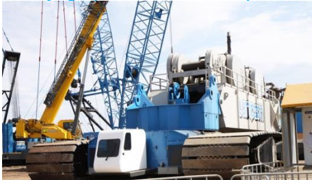
Assembly of the 2600 tonne heavy lift crane commences. Lift capacity of 1084 tonnes at 41 metre radius.
