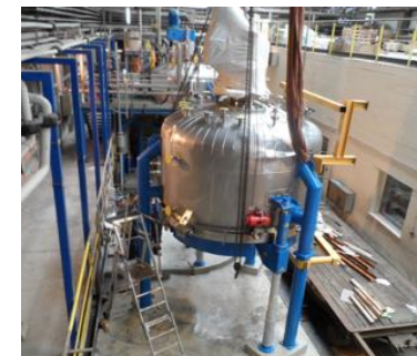
Auby : New filter is put in place. The filter is part of critical infrastructure for the recovery of valuable Indium metal.
